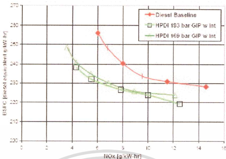
Trade-off between fuel consumption and NO x emissions for natural gas and diesel fueling. 8.96 bar BMEP, 1260 RPM.
