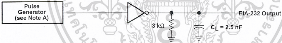
Figure 2. Driver Test Circuit and Waveforms for t_{PHL} and t_{PLH} Measurements (5- \mu s Input)
