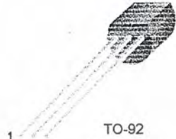
TO-92 1. Collector 2. Base 3. Emitter
