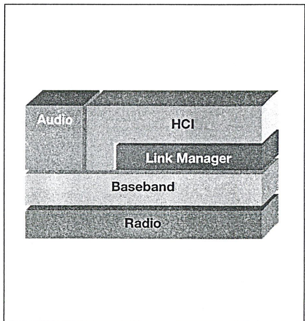
Figure 7. HW/FW parts included in the Ericsson Bluetooth module.
