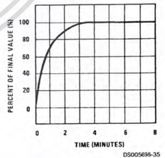
Thermal Response in Still Air
