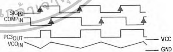
Figure 8. Typical Waveforms for PLL Using Phase Comparator 2
