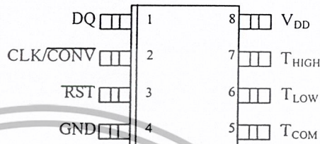
DS1620S 8-Pin SOIC (208-mil) See Mech Drawings Section
