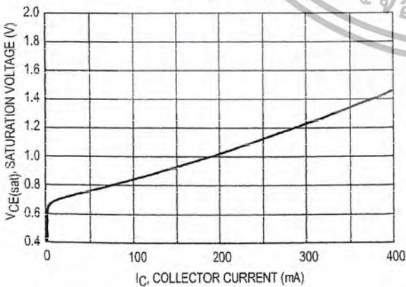
Figure 8. Common-Emitter Configuration Output Saturation Voltage versus Collector Current
