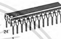
P SUFFIX PLASTIC PACKAGE CASE 724
