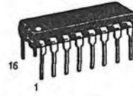
P SUFFIX PLASTIC DIP CASE 648
