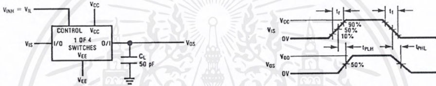
FIGURE 4. t_{PHL} , t_{PLH} Propagation Delay Time Signal Input to Signal Output
