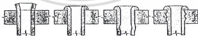
rolled and flared, rolled and beaded, expanded by prosser method, grooved tube seat
