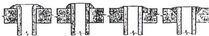
seat welded bead, rolled and welded, rolled and recess welded, rolled and bevel welded
