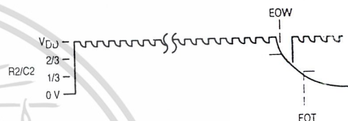
Figure 16. R-C Decay on Pin 10 (R2/C2)
