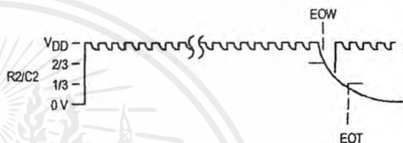
Figure 16. R-C Decay on Pin 10 (R2/C2)
