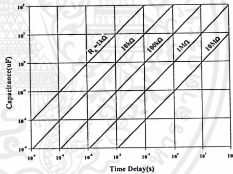
Figure 2. Resistance and Capacitance vs. Time delay(td)
