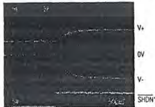
V+, V- WHEN EXITING SHUTDOWN (1µF CAPACITORS)
