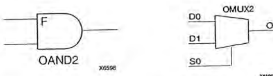
Figure 20: AND & MUX Symbols in XC4000X IOB
