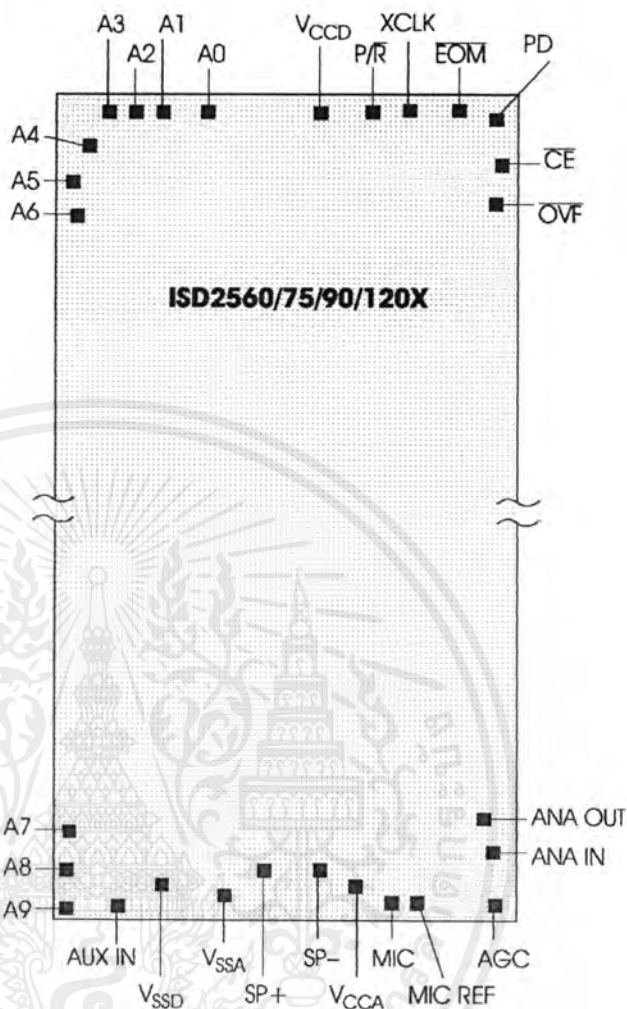
Figure 13: ISD2560/75/90/120 Products Future Bonding Physical Layout 1 (Unpackaged Die)
