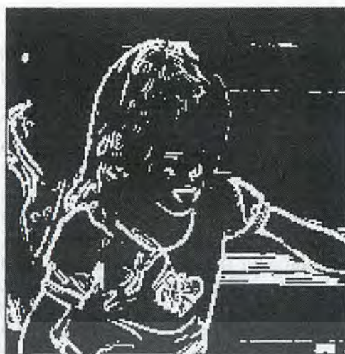
c. Edge detection and threshold operation.
