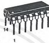
P SUFFIX PLASTIC PACKAGE CASE 646
