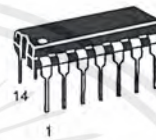
P SUFFIX PLASTIC PACKAGE CASE 646
