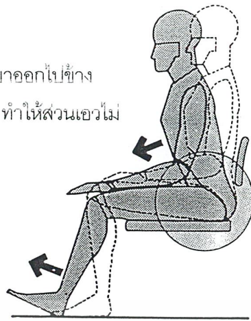
Figure 4-6. A seat surface located too low may cause the legs to become extended and positioned forward, depriving them of any stability. In addition the movement of the body forward will also cause the back to slide away from the backrest and deprive the sitter of proper lumbar support.
