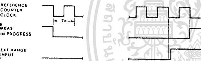
Abbildung 4: External Range Input und Measurement in Progress.
