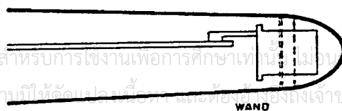
Figure 12-4. Apertured emitter sensor light pen
