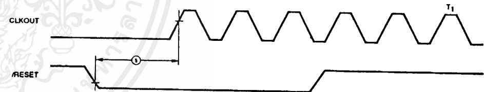
(b) Clock Restart Timing By /RESET (IDLE1/2 Mode)
