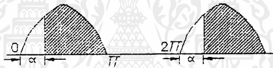
(c) Load Waveshape with Delay Angle ' ' - Natural Commutation
