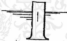
BELLMOUTH PIPE SUSPENDED IN BODY OF WATER, WITH ADEQUATE SUBMERGENCE AND CLEARANCE K = 0.2 (well rounded) TO 0.5 (slightly rounded)
