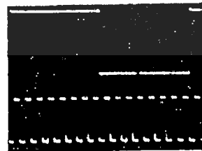
Figure 23. Typical Input/Output Waveforms For N = 16 Top: Input (100 kHz) Bottom: VCO Output (1.6 MHz) Vertical Scale 1 V/cm
