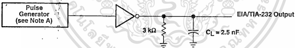
Figure 3. Driver Test Circuit and Waveforms for t_{PHL} and t_{PLH} Measurement (5- \mu\text{s} input)
