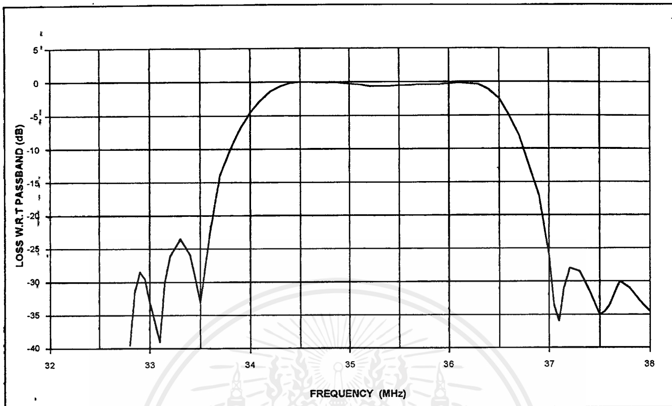
Fig.15 Typical frequency response of DW9255 SAW filter used as 2nd IF filter
