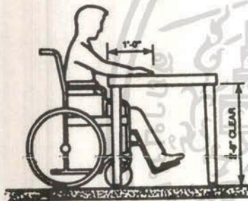
Fig. 3 Clearance under table.
