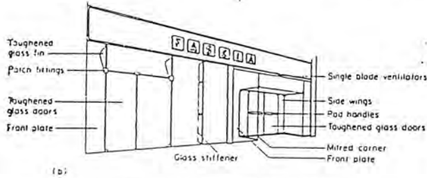
Shop fronts (a) Perspective showing components of typical shop front All glass construction to shop front
