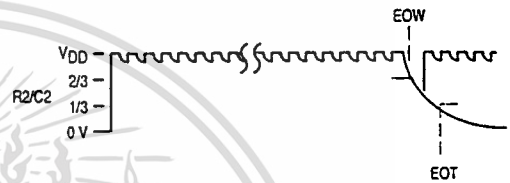
Figure 16. R-C Decay on Pin 10 (R2/C2)
