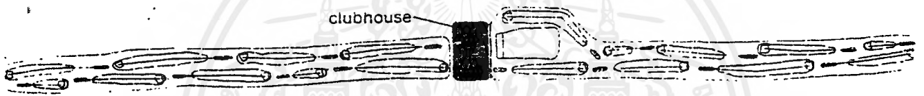
Figure 5.111 Double-fairway eighteen-hole course with returning nines. The course covers 150 acres, the minimum width between developed areas is 500 feet, and the length of the lot frontage is plus or minus 24,200 feet.
