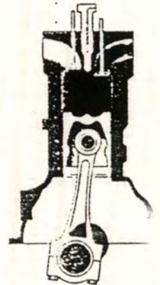
4 Piston reaches bottom and rises as exhaust valve opens, gases escape.
