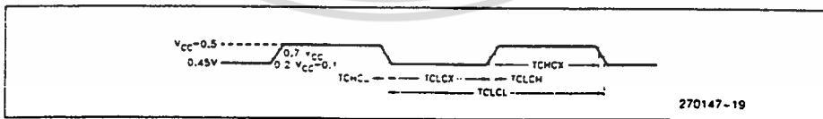
Figure 8. Clock Signal Waveform for I_{CC} tests in Active and Idle Modes. TCLCH = TCHCL = 5 ns.
