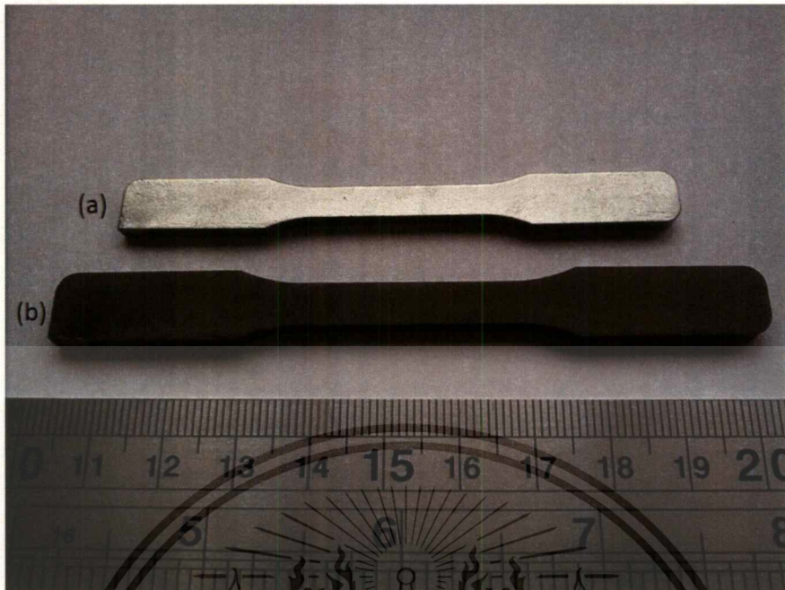
Figure 4.9 The figure of sintered (a) and green W-(Ni-Cu-Co) specimen (b).
