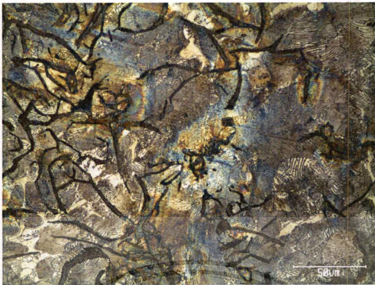
Figure 3.10 Microstructure of cylinder wall specimen (500X)
