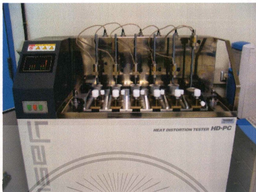
Figure 3.9 HDT/VICAT softening temperature tester (Yasuda model HD-PC)
