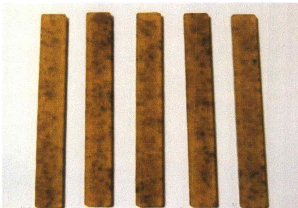
Figure 3.5 Flexural specimens testing
