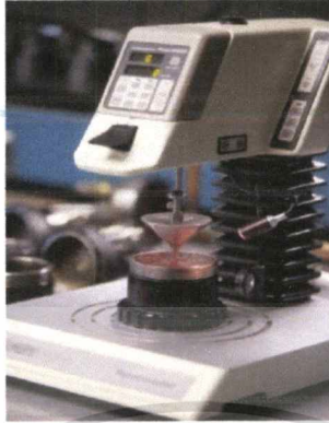
Figure 3.3 Apparatus for cone penetration of lubricating grease
