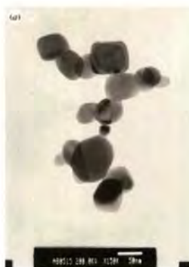
Figure 2.9 TEM of CuO nanoparticles (QinetiQ Nanomaterials Ltd) [80]
