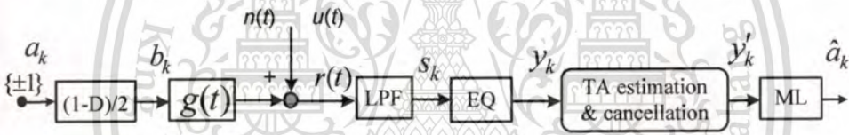
Figure 5.1 The magnetic recording channel model used in the simulation.
