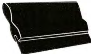
Figure 3.8 Screen printing brush was used for thinning the photoresist film
