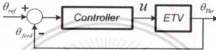
Fig. 5.2 SISO feedback control strategy for ETV control
