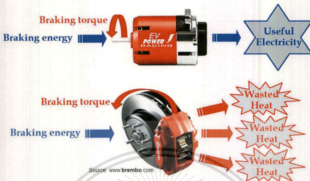
Figure 2.7 Comparison of regenerative and friction braking system
