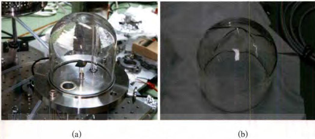
Figure 3.10 Pyrex® bell jar after using as the plasma chamber for 30 min.
