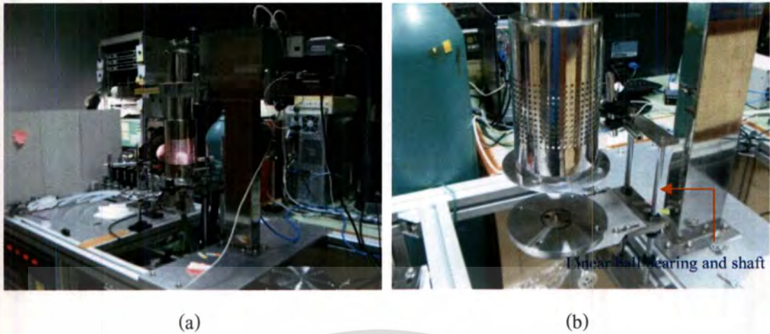
Figure 3.8 Photograph of the last version of the MPECVD apparatus (a) and the baseplate fixed to a linear ball bearing and shaft (b).
