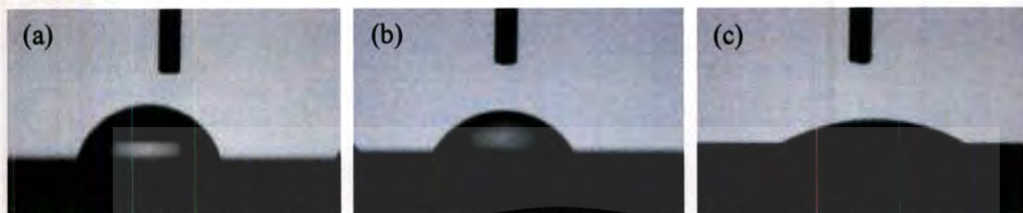
Fig. 2. Images of deionized water contact angle on Si substrate surfaces under various pretreatment methods: (a) mirror polish, (b) ultrasonic scratch, and (c) mechanical scratch.
