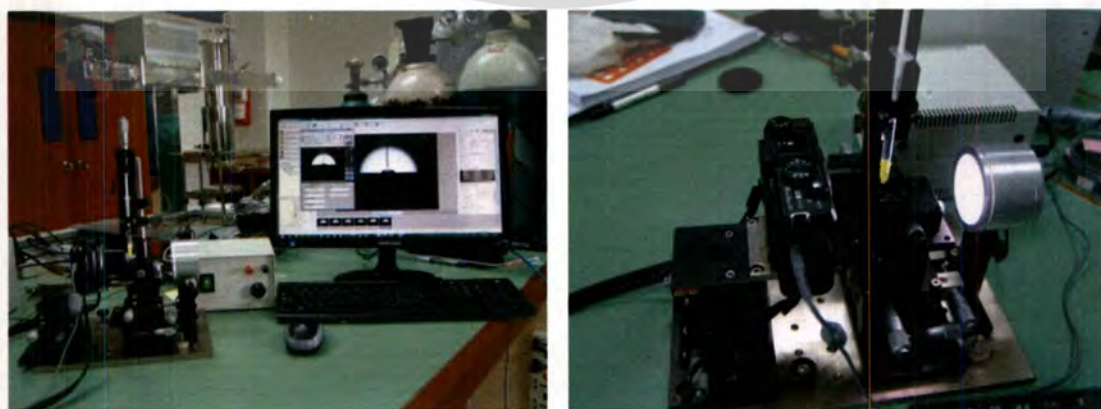
Figure 3.28 Contact angle measuring instrument with a laboratory setup.
