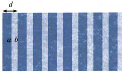
Figure 2.2 The schematic of the one-dimensional PBG structure.
