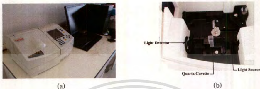
Figure 3.4 (a) The UV/VIS spectrometer and (b) Inside view of spectrometer box.
