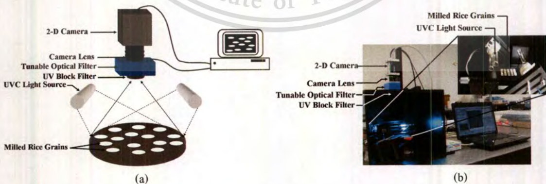
Figure 4.12 Experimental setup for KDML105 milled rice breed identification: (a) diagram and (b) perspective view.
