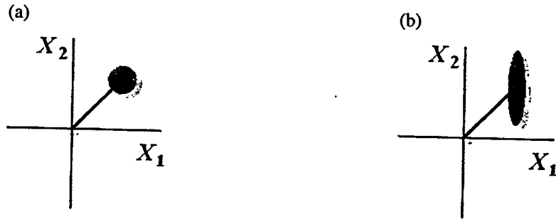
Figure 2.1 Phase-space plot showing the uncertainty in (a) a coherent state |\alpha\rangle , and (b) a squeezed state |\alpha, r\rangle .
