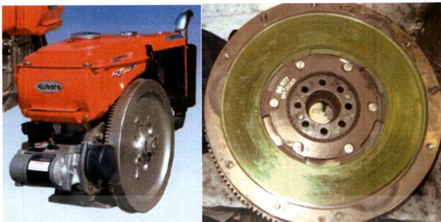
Figure 3.6 Flywheel comparison (Left) one cylinder diesel engine flywheel (Right) conventional engine flywheel (Clutch disc contact surface : Green area)
