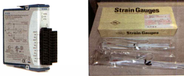
Figure 4.27 (left) Data acquisition tool NI-9235, (right) uniaxial TML strain gauges
