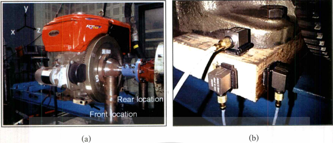
Figure 4.2 (a) accelerometer attach locations (b) accelerometers attachment configuration near engine base.
